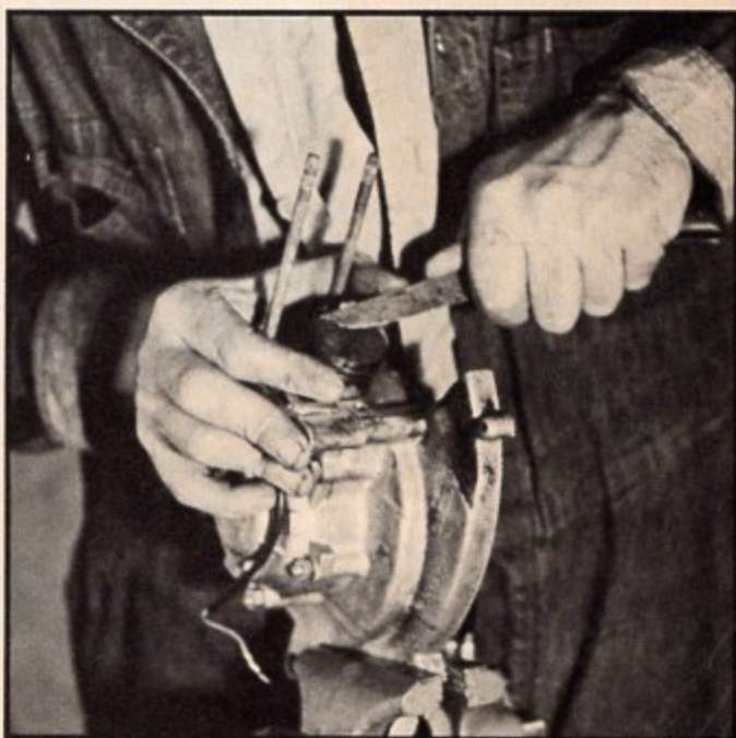
The piston head is particularly easy to work on with a knife blade. The coke just scrapes right off and your working on a surface you can control.
