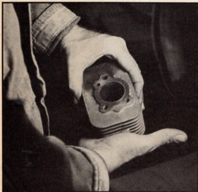
With the cylinder head removed, you may notice some carbon deposits building up on the head itself. You'll want to remove the crud with a rag, knife blade or brush.
