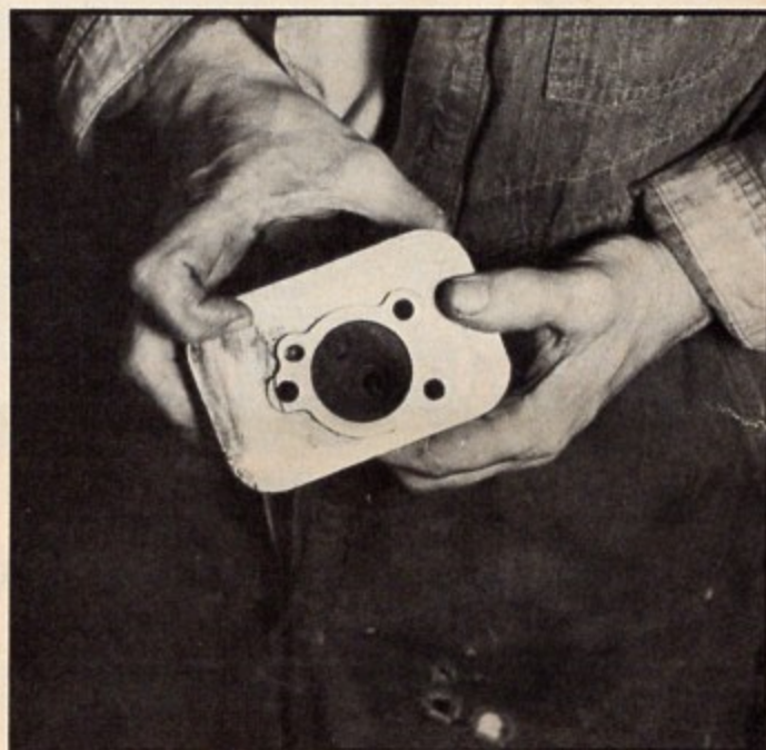
Once you've adequately removed the build-up, the head should give you a much brighter and smoother surface to look at.
