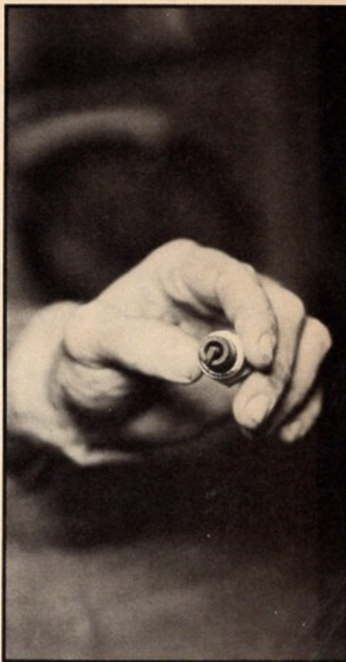
Check the plug for signs of coke deposits. You might want to gap the plug at this time, too.
