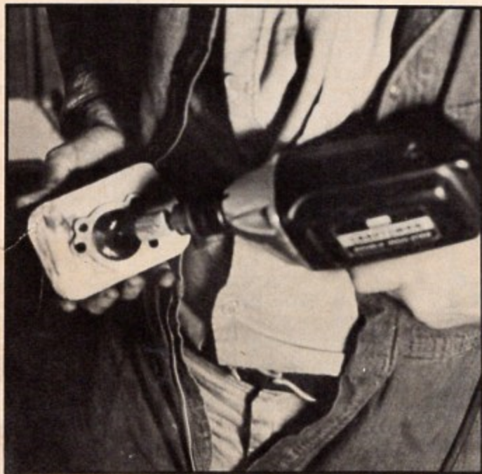
To get the coke inside the head, a brush, rat-tail file, pen-knife or grinder attachment for your drill can be used.
