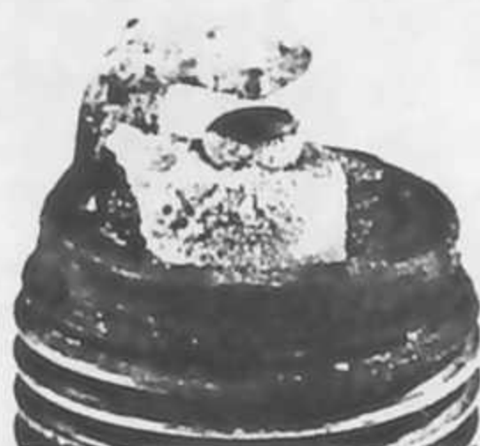
White deposits have accumulated from excessive amounts of oil in the combustion chamber or through the use of low quality oil. Remove deposits or a hot spot may form
