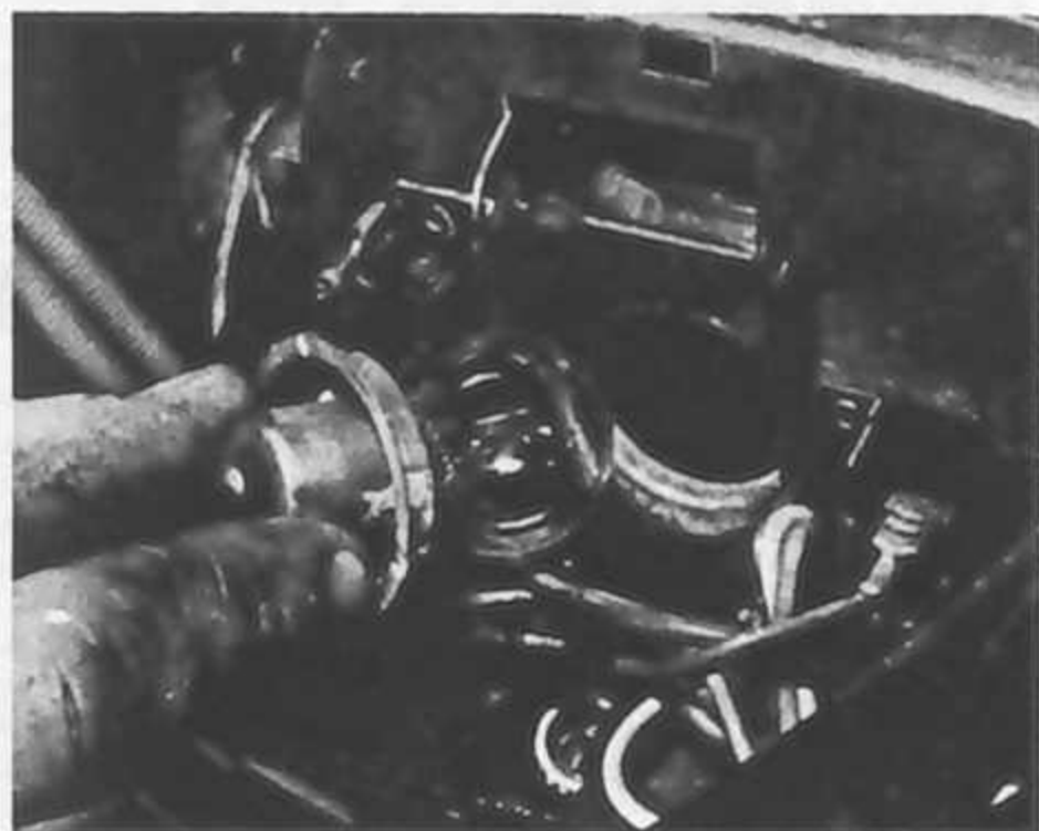
Displace contact to release headlamp bulb
