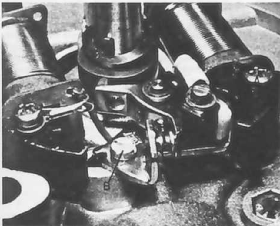
4.2 A: Lead securing screw. B: Fixed contact securing screw
