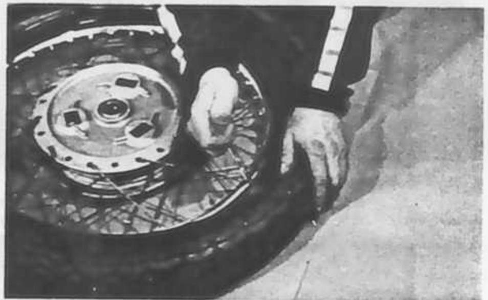
Work first bead over rim, using lever in final section
