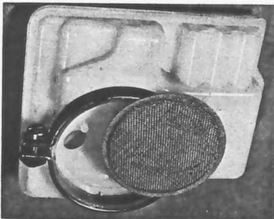
9.2 Clean filter element in petrol to remove dust
