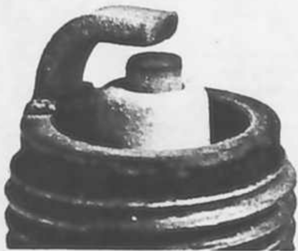
Spark plug conditions: A brown, tan or grey firing end is indicative of correct engine running conditions and the selection of the appropriate heat rating plug
