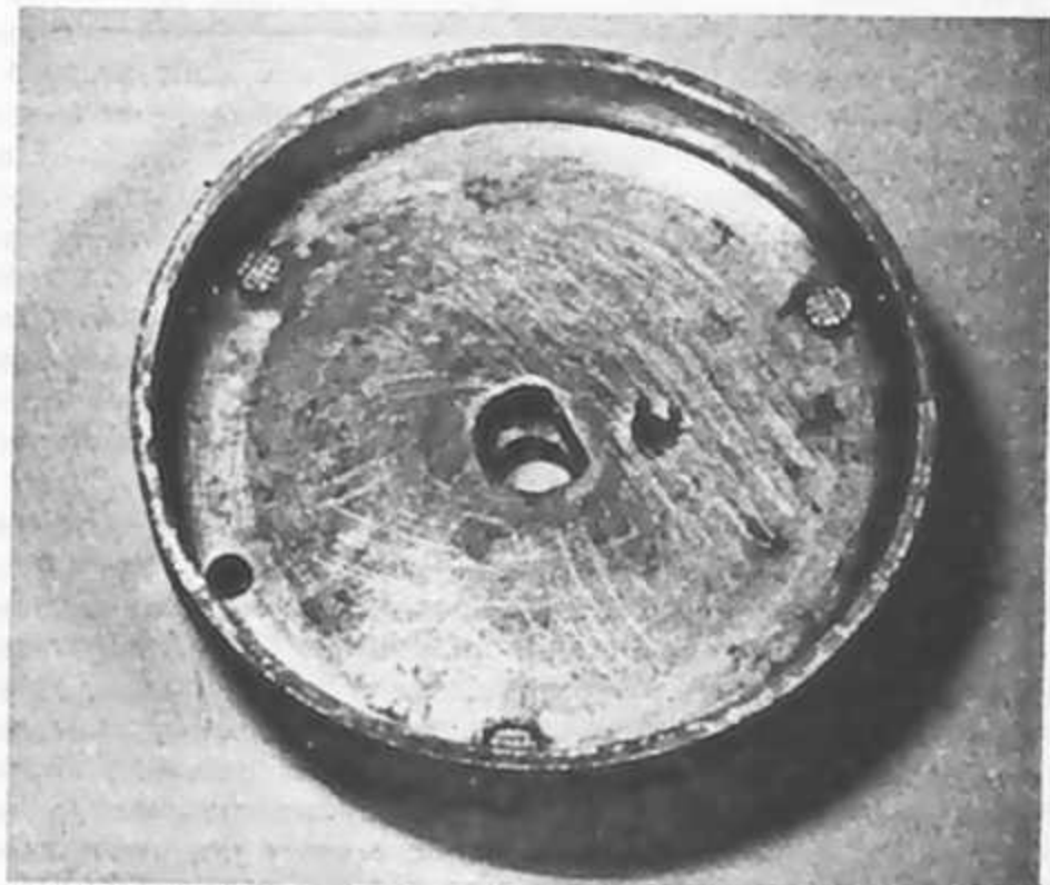
23.4b Backplate forms drum for starting shoes
