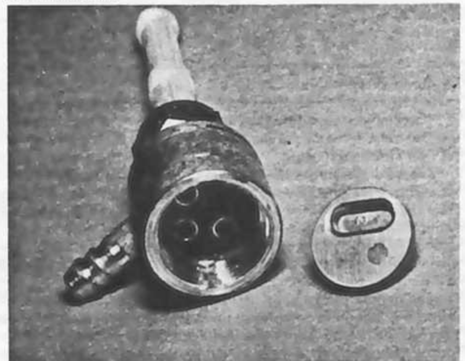
4.2b Petrol is channelled through slot in aluminium block
