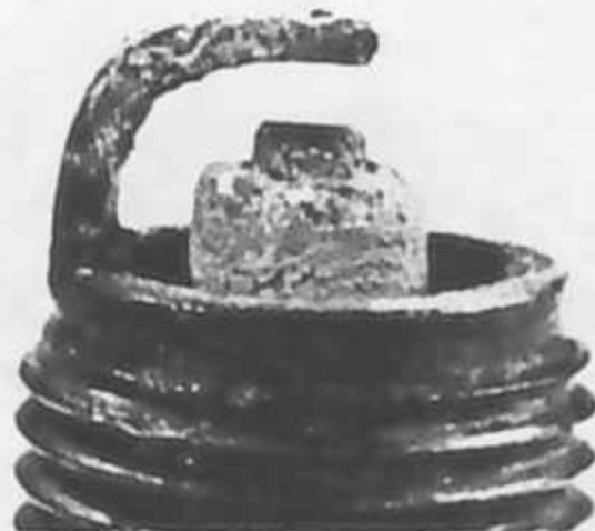
A worn spark plug not only wastes fuel but also overloads the whole ignition system because the increased gap requires higher voltage to initiate the spark. This condition can also affect air pollution
