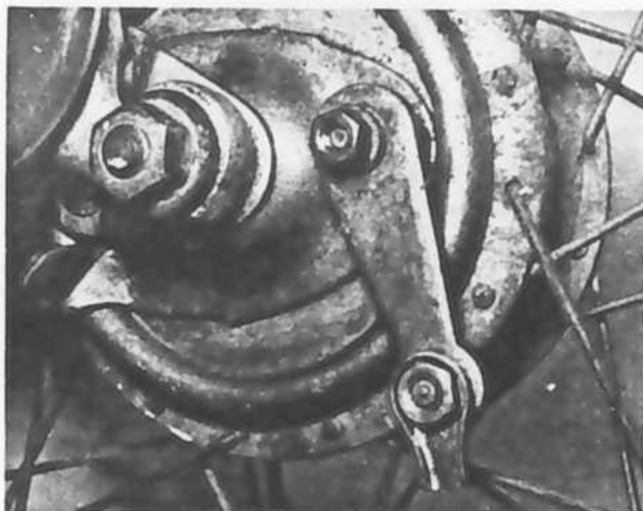
3.2 Release front brake cable and wheel nuts
