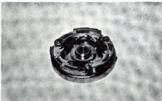
Fig. 70: When it becomes necessary to replace the clutch housing bearing, the housing should be heated to 80-90 degrees Centigrade, 176-194 degrees F. Once the above checks have been completed, the engine can then be assembled.
