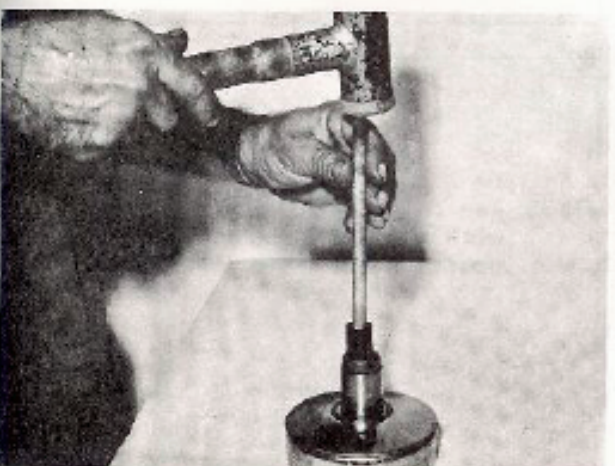
Fig. 58: Using the special tool #11, tap out the bearing and bushing.
