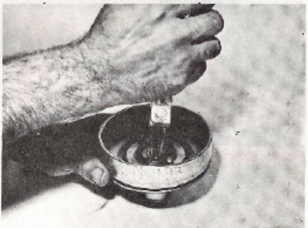
Fig. 57: To remove the clutch center bushing and bearing, first remove the large circlip.
