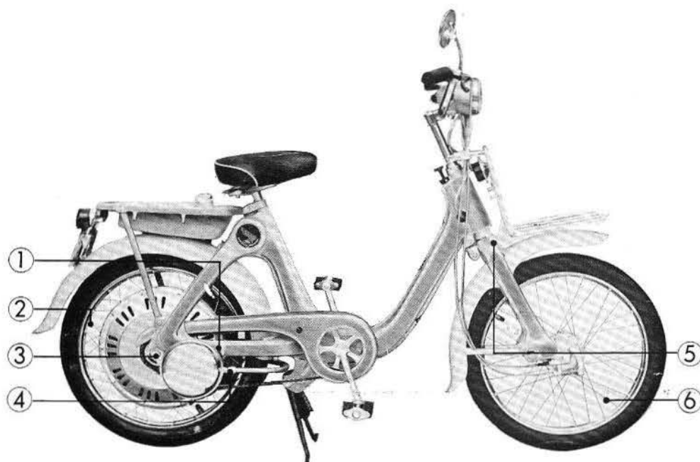
Fig. 1-25 ① 6x14 bolt ② Spoke ③ Rear axle nut ④ Muffler band ⑤ 6x14 screw (2 ea) ⑥ Spoke
