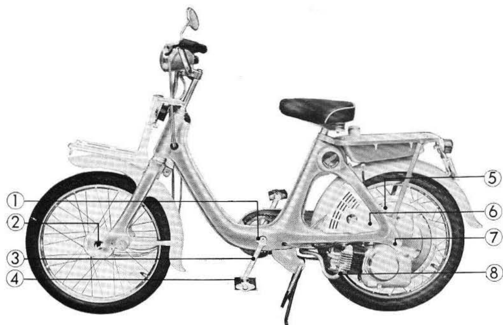
Fig. 1-24 ① Crank arm set pin ② Front wheel axle nut ③ Crank arm ④ Crank pedal ⑤ Rear torque arm ⑥ Carburetor cover ⑦ Rear axle nut ⑧ Exhaust pipe
